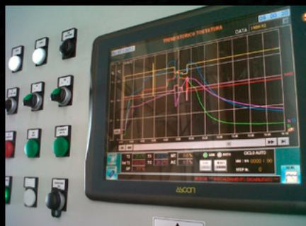
This control pack allows you to create total-flexibility roasting profiles through a modulating burner. It allows you to vary
